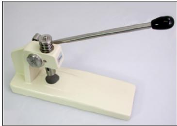
Sturdy, compact and easy To Use. The smooth action of the handle permits pellets to be pressed effortlessly with one hand and minimal pressure. Several different Die Sets (1mm, 3mm, 7mm) are available for use with the Table Press. The pellets are pressed using light operator pressure in a collar/die that can be transferred onto a pellet holder for transmission analysis.
